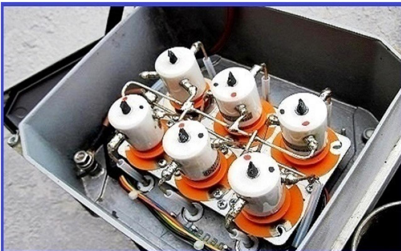
VERSIONE BOX REMOTO CON RELAYS SIEMENS VR421 di I2NOI
