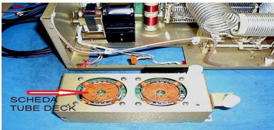
SCHEDA TUBE DECK NEL VANO PRESSURIZZATO SMONTATO
